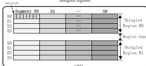
(b) Segment: A shingled region is further divided into segments in the radial direction. In each segment, the sectors in the same track constitute one block.
